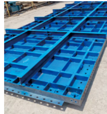
Base formwork 底模
